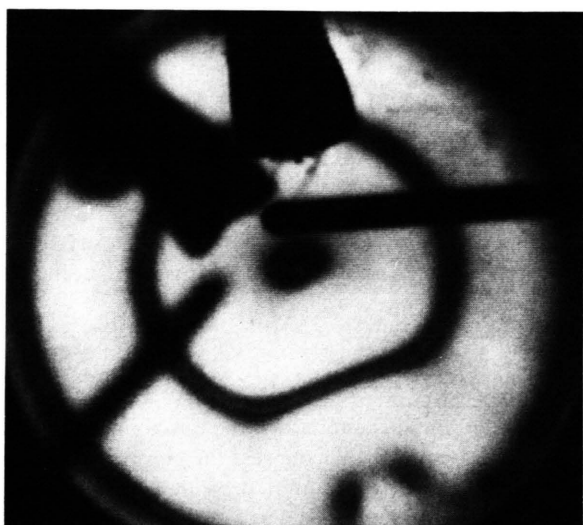
Fig. 5a. Fluid layer just after the pressure jump. The wavelength of the roll-shaped convective pattern is about two times the layer depth. The black shadows that are superimposed on the structures in this and the following pictures originate from the thermocouple and the jets inside the cavities (see Experimental). The disturbance in the lower part of the picture is caused by the fluid inlet of the sample cell.
